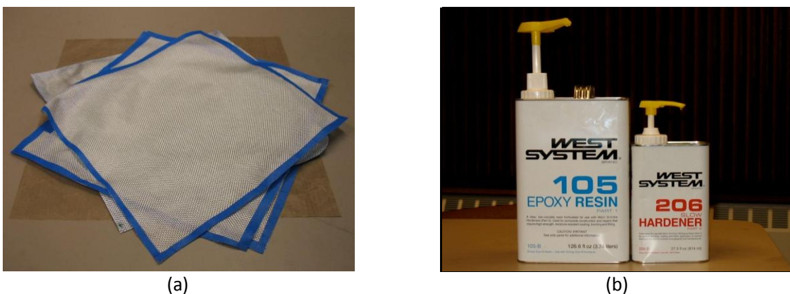
Figure 3. (a) woven fiberglass cloth stacked to illustrate layup (b) epoxy
